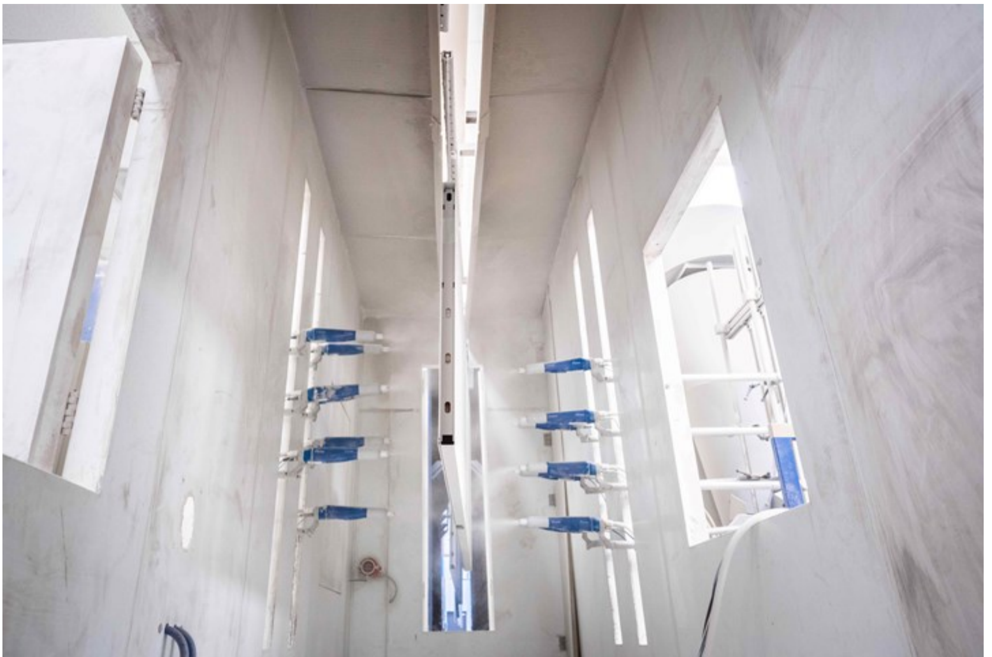
A door system being powder coated in a booth.
