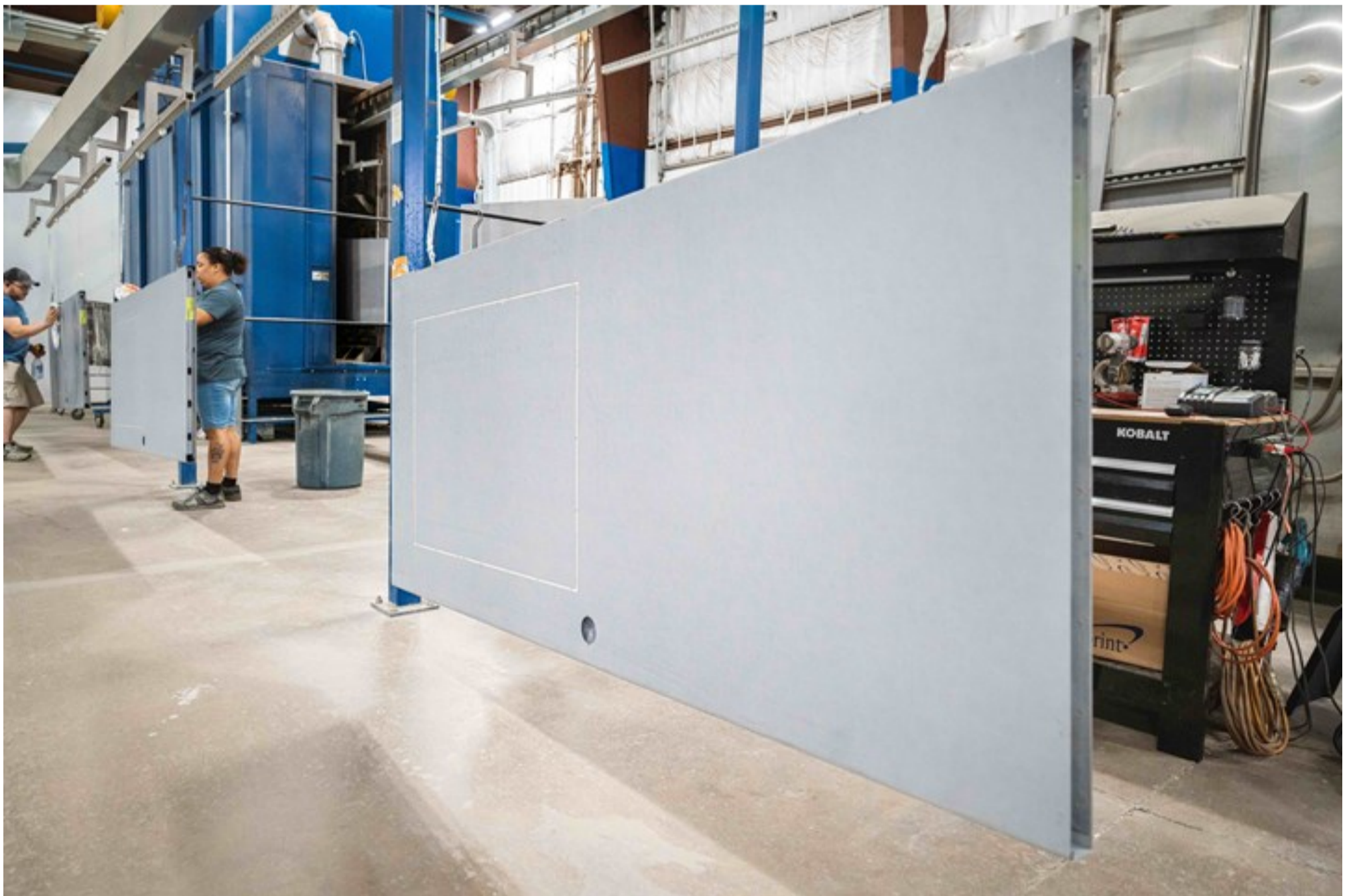
A door system waiting to receive treatment in the finishing line. Employees inspect other systems farther down. Photo Credit, all: Global Building Products
